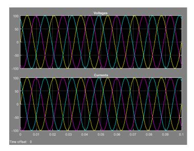
In this example, the **Component structure** parameter of the RLC block specifies that the electrical characteristics of the three-phase load are purely resistive. Therefore, for each phase of the three-phase system, the voltage and current remain in phase with each other. Because the resistance in each phase is  $1 \Omega$ , the magnitude of the phase voltage is equal to the magnitude of the phase current.
