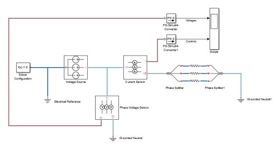
**9** Save this version of the modified model using the name simplethreephasemodel expanded balanced.
